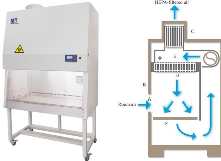
Figure 47. Graphic depiction Biosafety Cabinet and negative airflow with high-efficiency particulate (HEPA) filter
